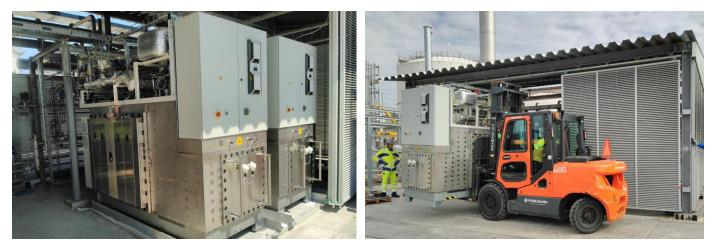
Pictures: Sunfire delivers two high-temperature electrolysis modules to Neste's renewable products refinery in Rotterdam.
